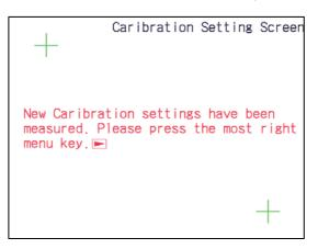
(4) Check whether the calibration settings have been successfully measured.
