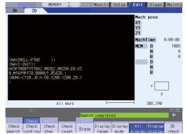
When the check search is completed, the graphic previously displayed is erased and the auto-adjustment of the scale will start.
