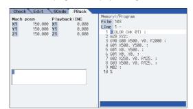
(Note 1) When the program is not displayed in the right area, a playback editing will not be executed. (Note 2) When the incremental value is set, playback movement amount will be cleared to 0 for all axes.
